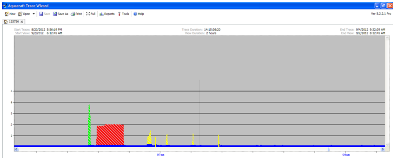
Figure 69: Two-hour view of 12S756. Leaks are blue, faucets are yellow, toilets are green, and showers are red.
