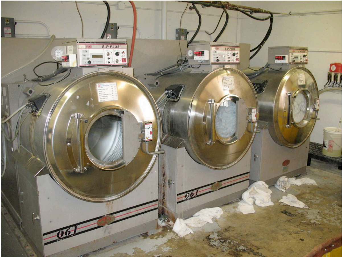
Figure D-1 Three Pellerin Milnor Model 36026Q6J 96 lb Capacity Washer-Extractors
