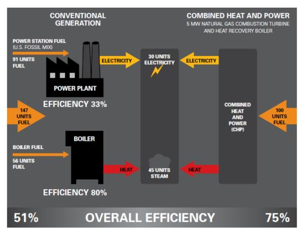
The NRDC graphic above was adapted from one developed by EPA, using all of the same input and output assumptions. EPA calls this an "example of a typical CHP system". As the analysis below shows, there is a reduction in *source* use of gas only if at least 50% of the reduction in grid electricity was produced by gas-fired power plants.
