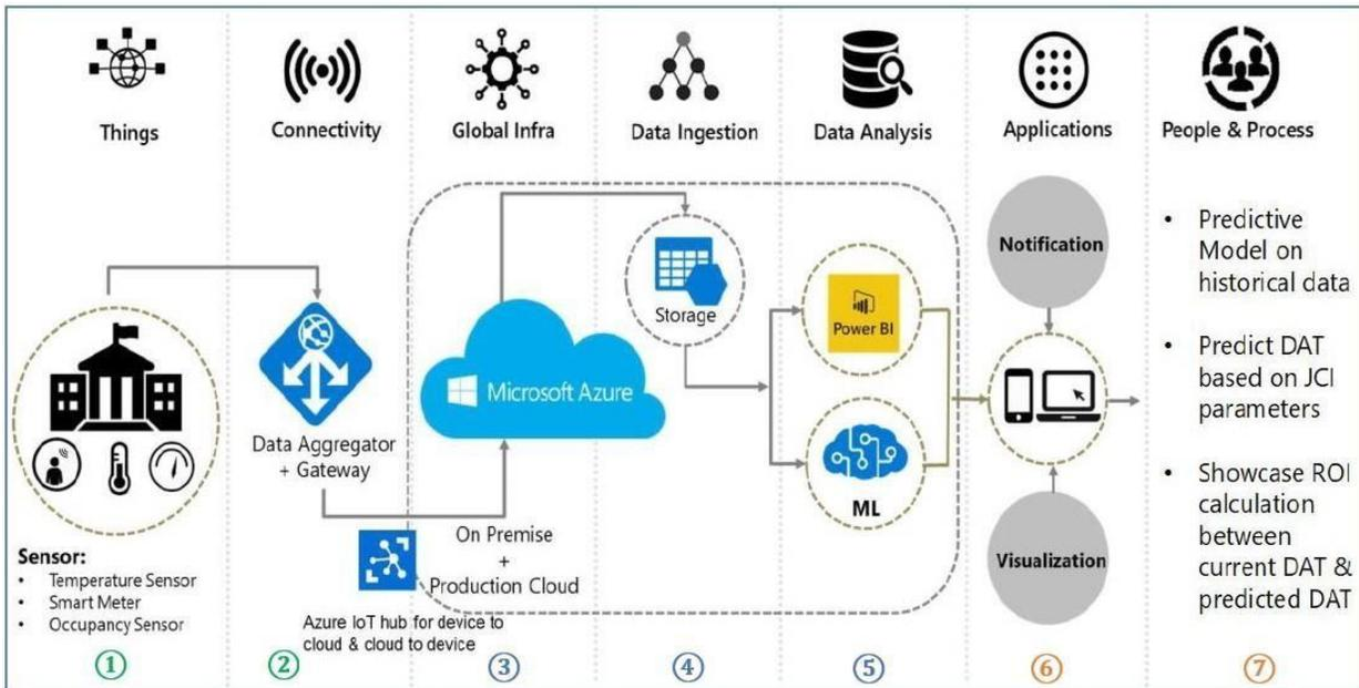
Figure 1: Optimized air handler system architecture. Green (1-2) represents layers located on-site at the Art Institute. Blue (3-5) represents layers located in the Azure Cloud, and orange (6-7) represents the user-facing layers accessible via the internet.
