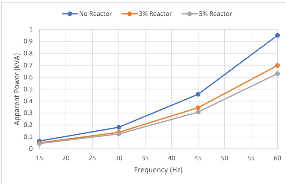
Figure 2. Apparent Power (kVA) Vs. Drive Speed
