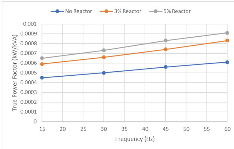
Figure 3. True Power Factor (kW/kVA) Vs. Drive Speed
