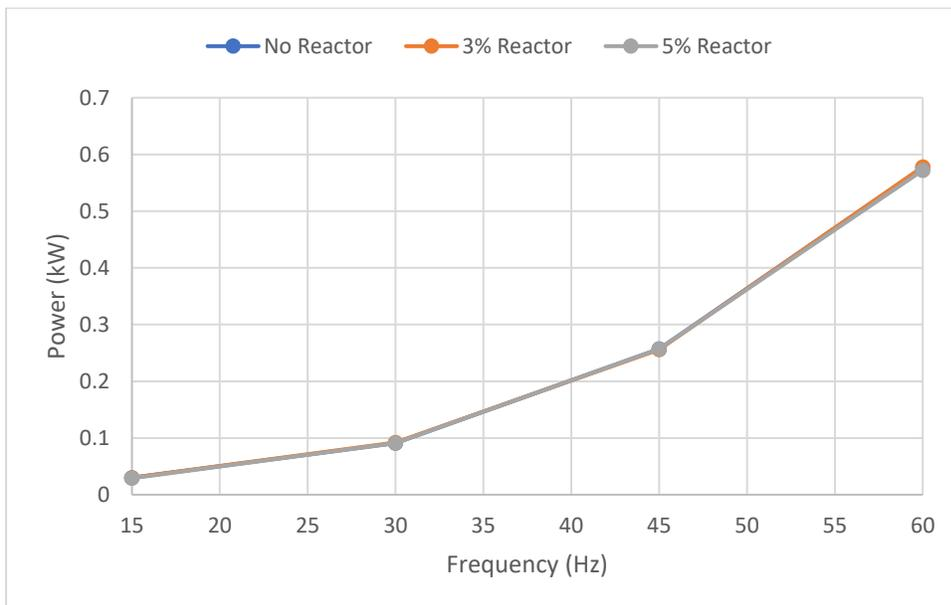
Figure 4. Real Power (kW) Vs. Drive Speed
