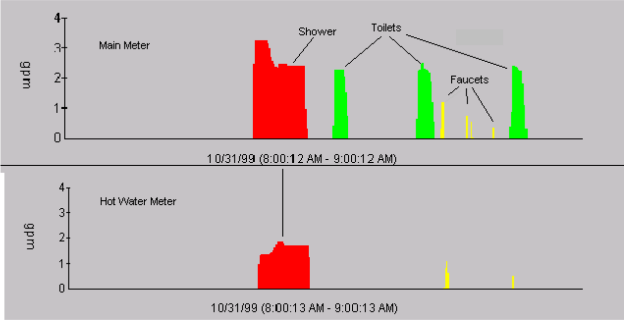
Figure 1: Simultaneous Flow Traces from Main (top) and Hot Water (bottom) Meters
